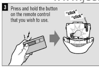
Release the button when the garage door opener lights blink **or** two clicks are heard. If programming to other products, press the button a second time to activate the product.
